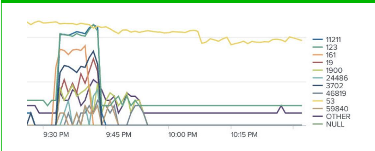
MULTIPLE UDP REFLECTION VECTORS BY SOURCE PORT IN A 15 MINUTE CARPET BOMB ATTACK
